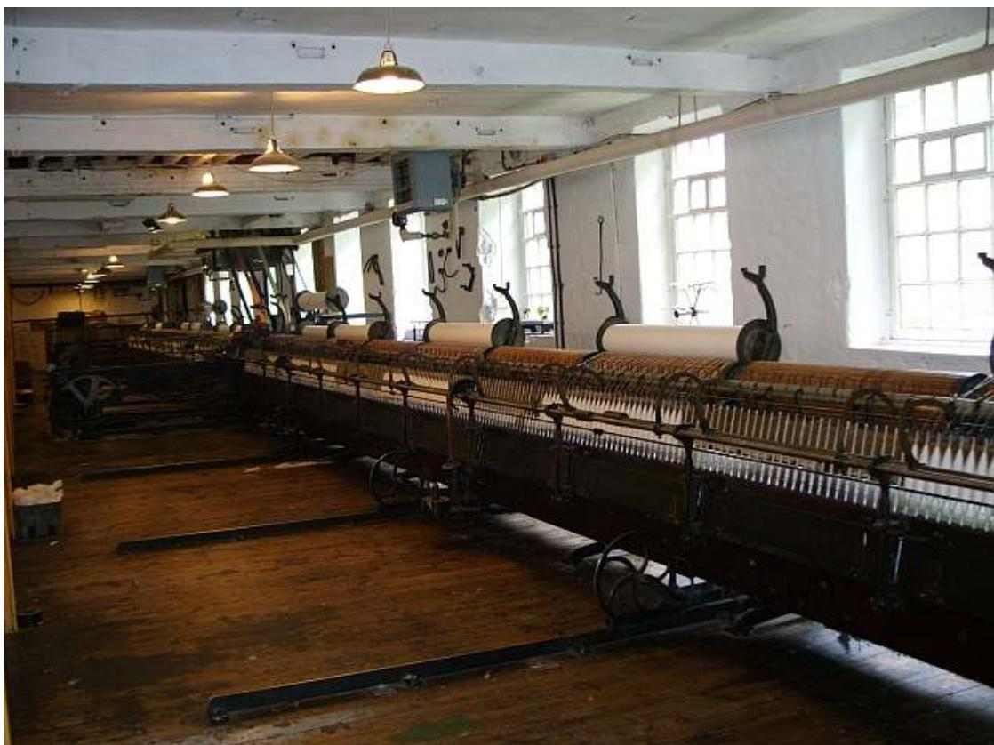
*A working Mule spinning machine at Quarry Bank Mill*
